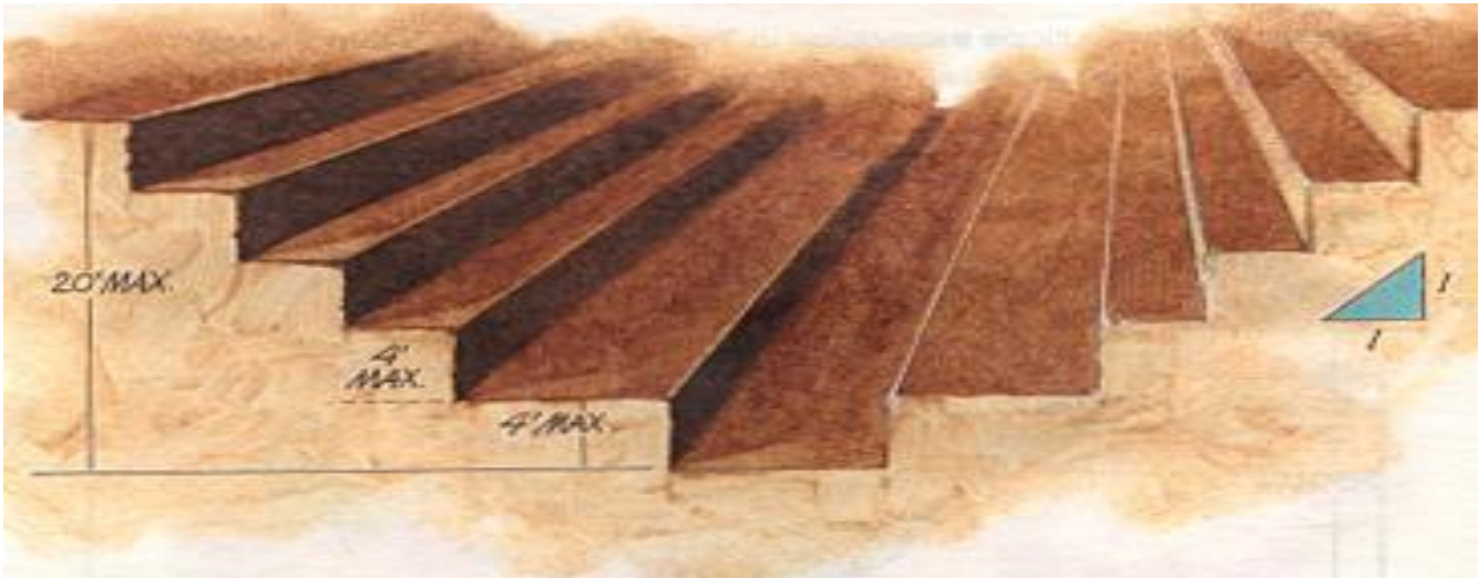
Figure 44: Stepped benched excavations
